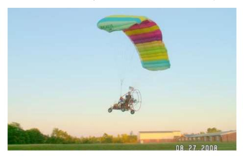
Flying the craft requires a Sports Pilot License. It is rated to 10,000 feet altitude, nominal altitude is 2,500 feet. Climb rate is 600 ft/min and has a 10-gallon fuel tank. During operation it uses 3-3.5 gal/hr. Therefore flight time can be in the range of 1-1.5 hours.
